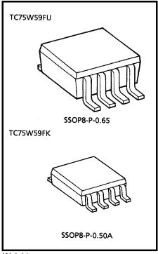
Weight SSOP8-P-0.65: 0.021g (typ.) SSOP8-P-0.50A: 0.01g (typ.)
