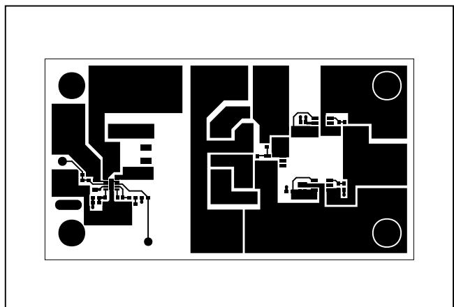
Figure 2. MAX17681V EV Kit PCB Layout—Component Side
