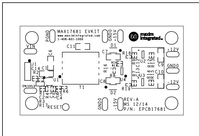
Figure 1. MAX17681 EV Kit Component Placement Guide—Component Side
