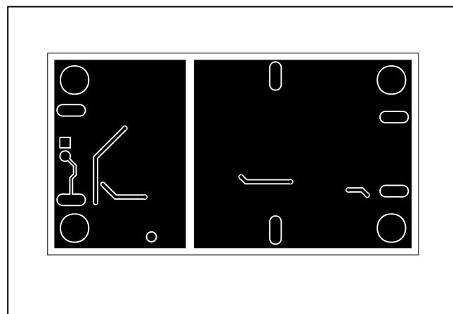
Figure 3. MAX17681 EV Kit PCB Layout—Solder Side
