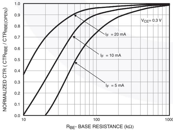
Figure 7. CTR vs. R<sub>BE</sub> (Saturated)
