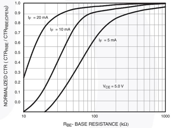
Figure 6. CTR vs. R<sub>BE</sub> (Unsaturated)
