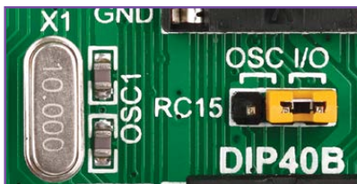
Figure 4-6: RC15 as I/O pin (when using internal oscillator)
