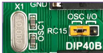
Figure 4-7: RC15 connected to X1 quartz-crystal
