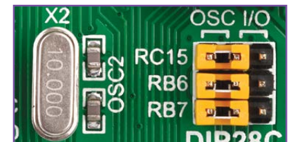
Figure 4-9: RC15, RB6 and RB7 connected to X2 quartz-crystal
