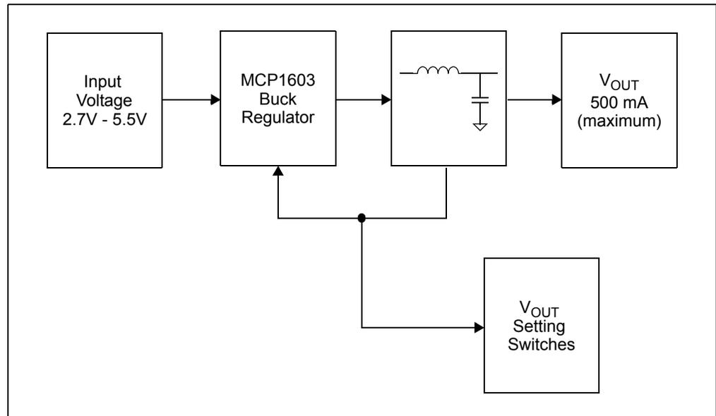
**FIGURE 1-1:** MCP1603 Buck Converter Evaluation Board Block Diagram.
