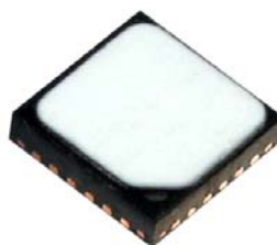
Figure 8. Si7005 with Factory-Installed Protective Cover
