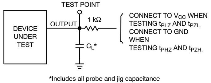
Figure 6. Test Circuit
