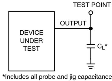
Figure 5. Test Circuit
