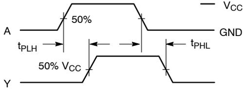
Figure 3. Switching Waveforms
