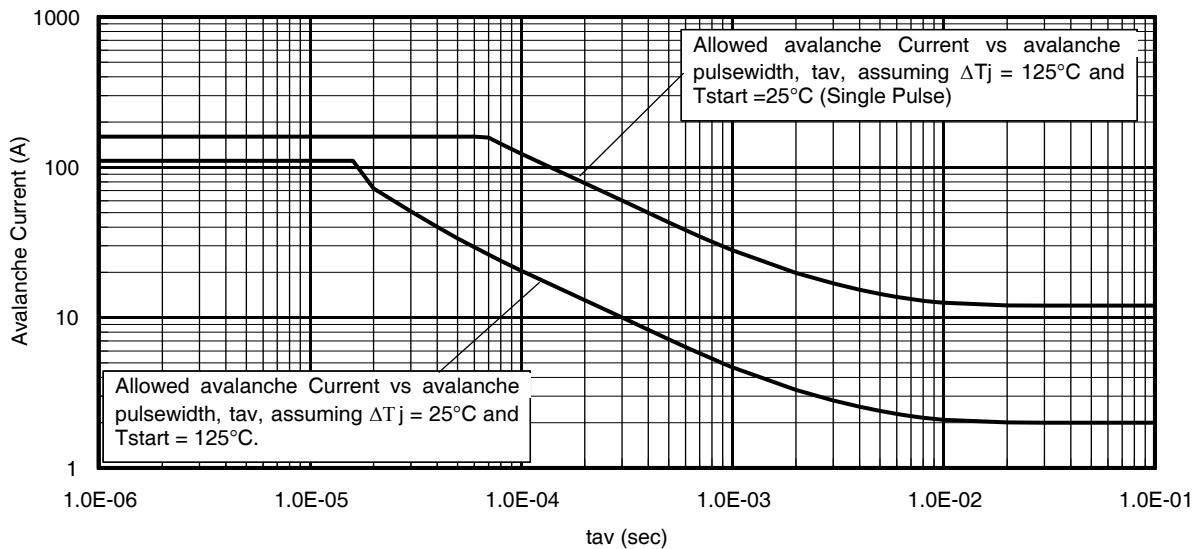
**Fig 14.** Single Avalanche Current vs. pulse Width
