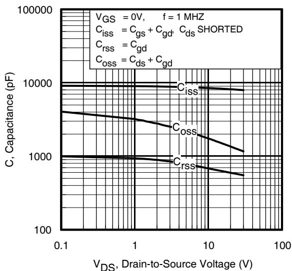
**Fig 5.** Typical Capacitance vs. Drain-to-Source Voltage
