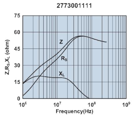
Impedance, reactance, and resistance vs. frequency.
