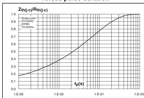
**Figure 4. Relative variation of thermal impedance junction to case versus pulse duration**
