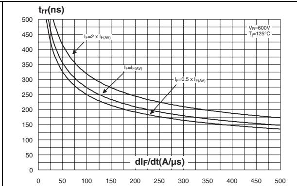
**Figure 7. Reverse recovery charges versus  $dI_F/dt$  (typical values)**
