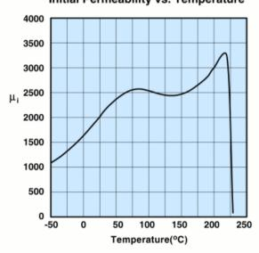
Measured on an 18/10/6mm toroid at 100kHz.
