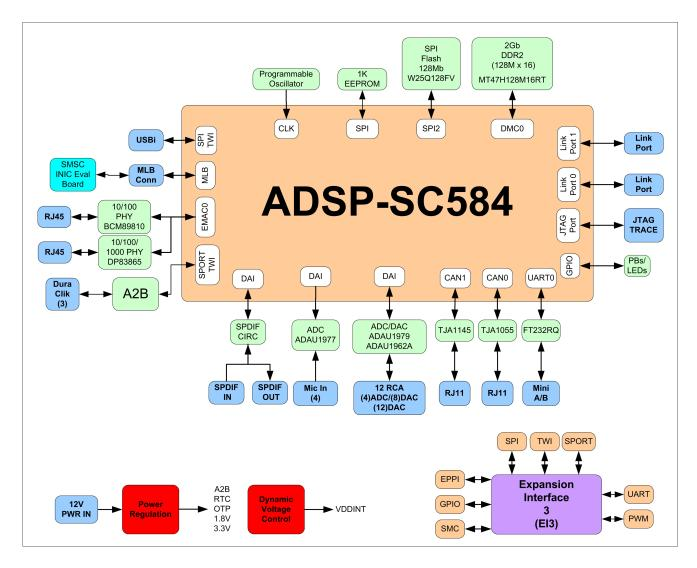
The ADSP-SC584 EZ-Board has two 25 MHz input clocks and runs at a max core clock frequency of 450 MHz. The input clock frequency can be changed through the SI5356A I2C programmable clock generator.
