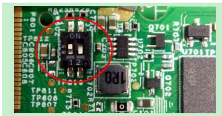
Figure 4. SW602 boot mode settings
