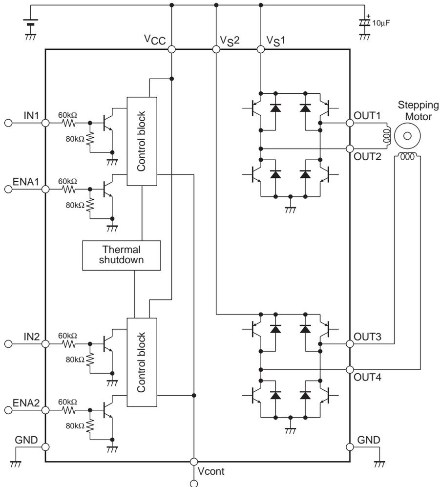
Note: As long as the voltages applied to VCC, VS1, VS2, ENA1, ENA2, IN1, and IN2 are within the limits set by the absolute maximum ratings, there are no restrictions on the relationship of each voltage level in comparison with the others (regarding which is higher or lower). (ex. VCC = 3V, VS1, 2 = 2V, ENA = IN = 5V)
