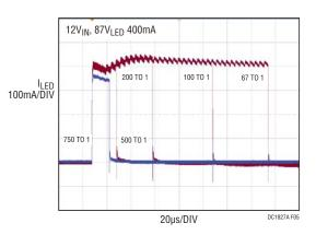
Figure 5. LED Current During PWM Dimming at 100Hz
