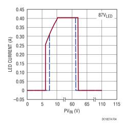
Figure 4. The LED String is 87V. This Output Current vs Input Voltage Graph Shows the Wide Input Voltage Range and the Input Voltages at Which UVLO, Turn-On and OVLO Occur. Input Current Limit Occurs When  $V_{IN}$  Is 10V or Less.
