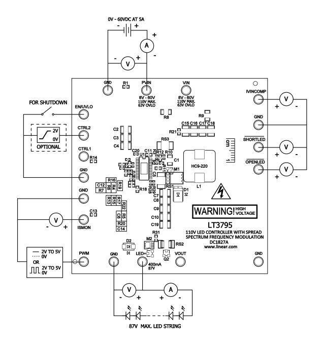
Figure 1. Proper Measurement Equipment Setup for DC1827A
