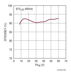
Figure 3. DC1827A Efficiency with 87V<sub>LED</sub> at 400mA
