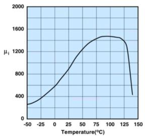
Measured on a 17/10/6mm toroid at 100kHz.
