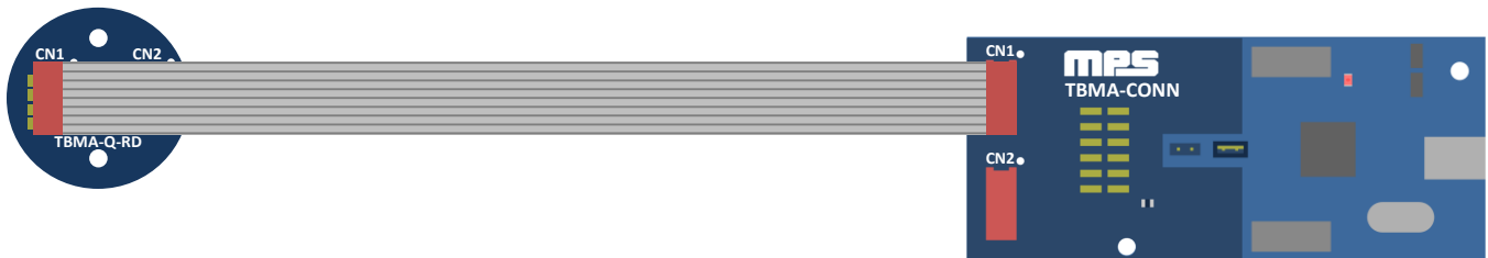
Figure 16: Connect TBMA-RD to TBMA-CONN Board
