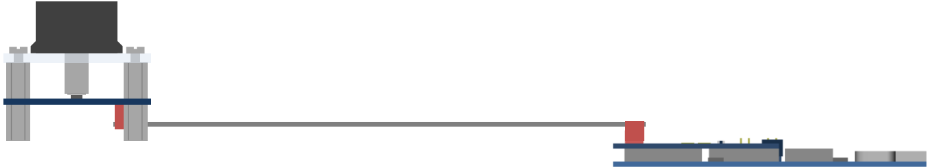
Figure 19: Connect EVKT-KNOB to EVMA-CONN Board (Side View)
