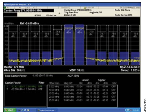
Figure 27. Two-Carrier W-CDMA at 875 MHz
