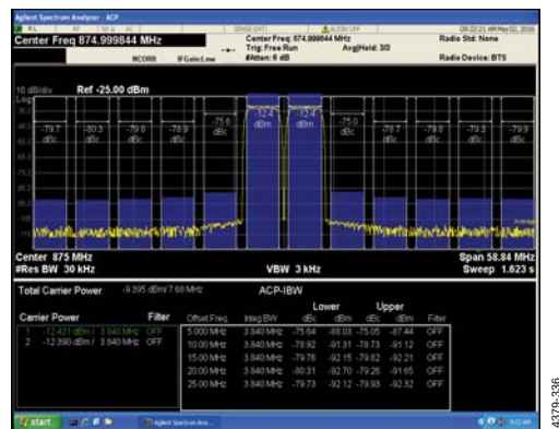
Figure 27. Two-Carrier W-CDMA at 875 MHz
