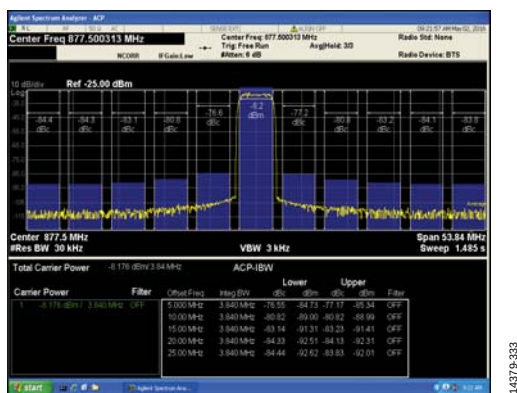
Figure 25. Single-Carrier W-CDMA at 877.5 MHz
