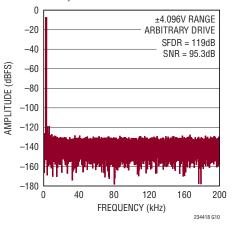
32k Point FFT f<sub>SMPL</sub> = 400kHz, f<sub>IN</sub> = 2kHz
