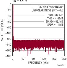
SNR, SINAD vs  $V_{REFBUF}$ ,  $f_{IN} = 2kHz$
