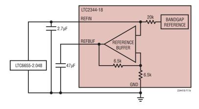
Figure 11b. External Reference with Internal Buffer Configuration
