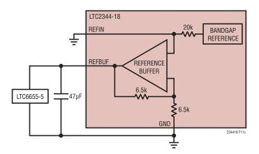
Figure 11c. External Reference with Disabled Internal Buffer Configuration
