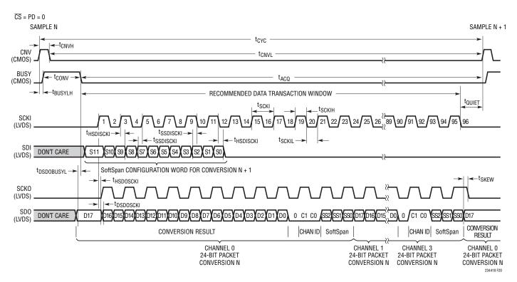
Figure 20. Serial LVDS I/O Mode
