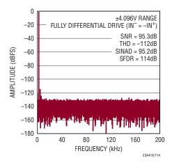
Figure 14. 32k Point FFT  $f_{SMPL} = 400ksps$ ,  $f_{IN} = 2kHz$
