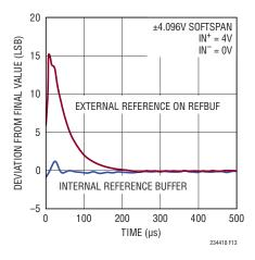
Figure 13. Burst Conversion Response of the LTC2344-18,  $f_{SMPL} = 400 \text{ksps}$
