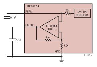
Figure 11a. Internal Reference with Internal Buffer Configuration
