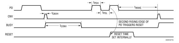
Figure 15. Reset Timing for the LTC2344-18
