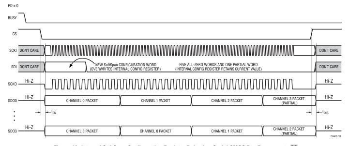
Figure 18. Internal SoftSpan Configuration Register Behavior. Serial CMOS Bus Response to CS
