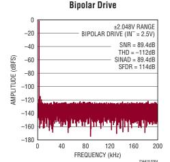
Figure 6d.  $IN^+ = -1dBFS$  2kHz Bipolar Sine,  $IN^- = 2.5V$ , 32k Point FFT, f<sub>SMPL</sub> = 400ksps. Circuit Shown in Figure 6a with LT6237 Amplifiers,  $R_{FILT} = 24.9\Omega$ ,  $C_{FILT} = 1nF$
