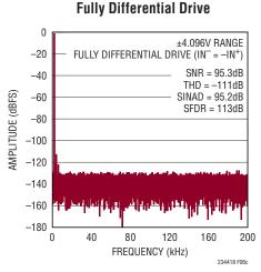
Figure 6c.  $IN^+/IN^- = -1dBFS$  2kHz Fully Differential Sine, Common Mode = 2.5V, 32k Point FFT, f<sub>SMPL</sub> = 400ksps. Circuit Shown in Figure 6a with LT6237 Amplifiers,  $R_{FILT} = 24.9\Omega$ ,  $C_{FILT} = 1nF$
