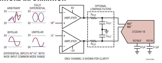
Figure 6a. Buffering Arbitrary, Fully Differential, Bipolar, and Unipolar Signals. See Table 2 For Recommended Amplifier and Filter Combinations
