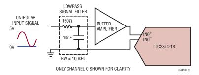
Figure 5. Unipolar Signal Chain with Input Filtering
