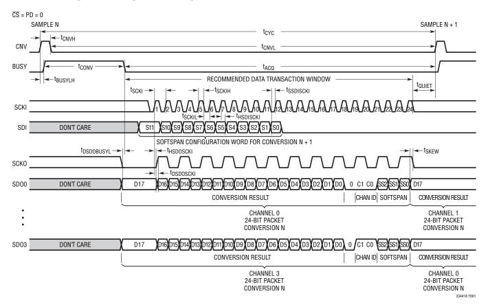
Figure 17. Serial CMOS I/O Mode
