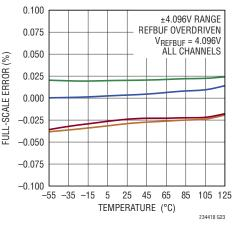
Negative Full-Scale Error vs Temperature and Channel
