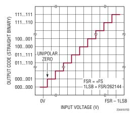
Figure 3. LTC2344-18 Straight Binary Transfer Function
