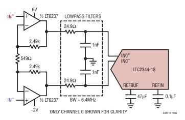
Figure 9a. Digitize Differential Signals with High CMRR
