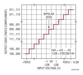
Figure 2. LTC2344-18 Two's Complement Transfer Function
