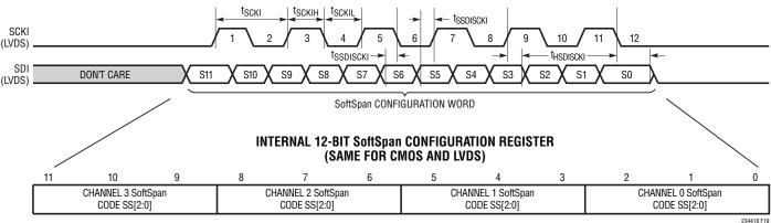
Figure 19. Mapping Between Serial SoftSpan Configuration Word, Internal SoftSpan Configuration Register, and SoftSpan Code for Each Analog Input Channel
