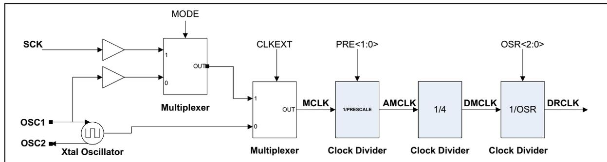
**FIGURE 4-1:** Clock Sub-Circuitry.
