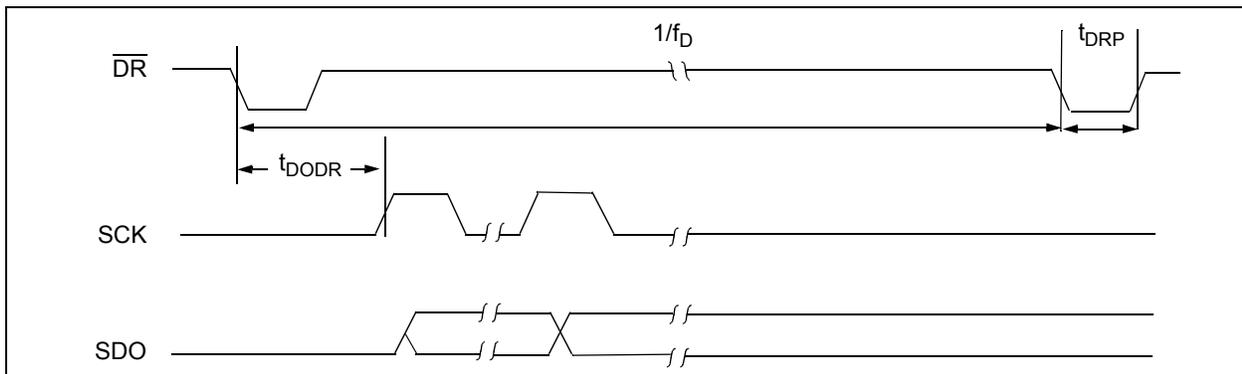
**FIGURE 1-3:** Data Ready Pulse / Sampling Timing Diagram.
