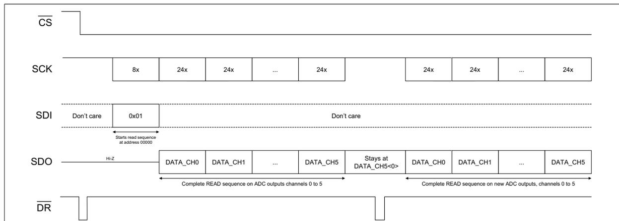
**FIGURE 6-8:** Typical Continuous Read Communication (WIDTH\_DATA<1:0> = 01, SPI Mode 1,1).
