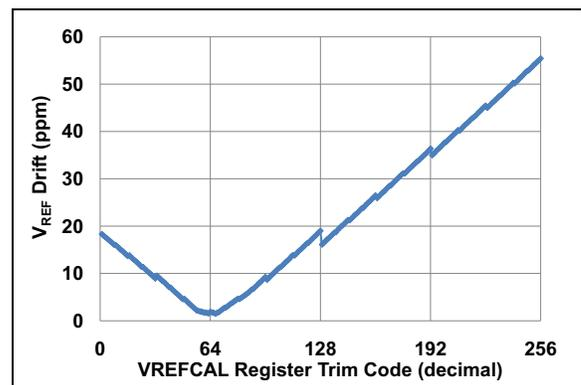
**FIGURE 5-6:**  $V_{REF}$  Tempco vs.  $V_{REFCAL}$  Trim Code Chart.
