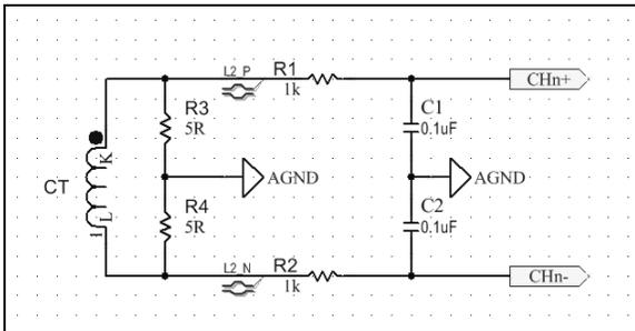
**FIGURE 7-6:** First-Order Anti-Aliasing Filter for CT-Based Designs.
