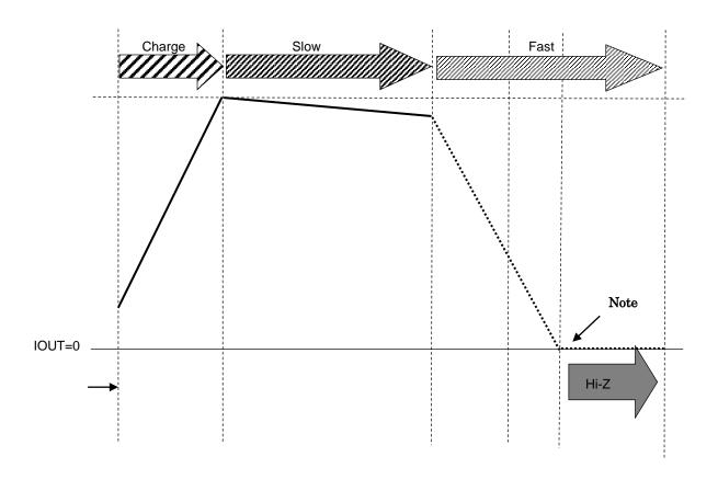
Note: When the motor current reaches the 0A level, the output transistor will turn to "Hi-Z" status.
