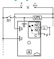
V = Voltage S1 = Initiate Switch L = Timed Load UTL = Untimed Load (optional) NO = Normally Open C = Common, Transfer Contact
