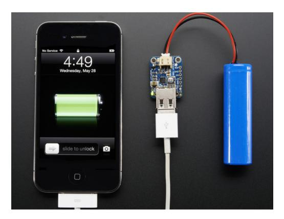
Great for powering your robot, Arduino project, single-board-computer such as Raspberry Pi or BeagleBone! Each order comes with one fully assembled and tested PCB and a loose USB A jack. If you are powering your project from USB, solder the USB A jack in (a 3-minute soldering task). If you would like to use a terminal block, pick up a 3.5mm 2pin block here (https://adafru.it/duR) and solder to the output spot where the USB jack would go. Or dont solder anything in for a more compact power pack.
