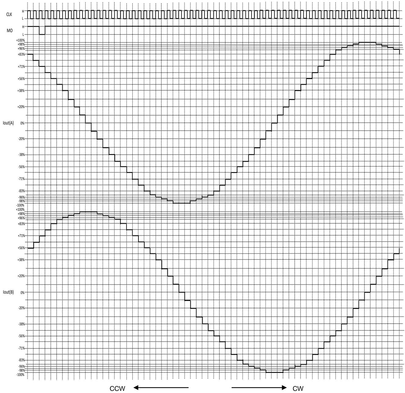
MO output shown in the timing chart is when the MO pin is pulled up.
