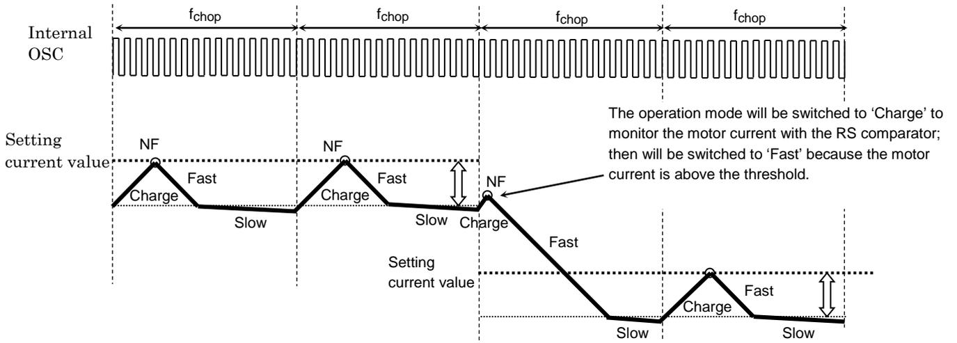
•When the Fast continues past 1 fchop cycle (the motor current not reaching the ADMD threshold during 1 fchop cycle)
