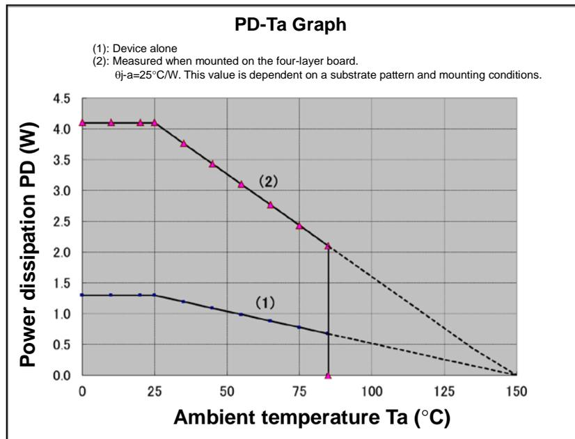
\* This value is dependent on a substrate pattern and mounting conditions. Please be careful. Moreover, power dissipation becomes small when ambient temperature is high.
