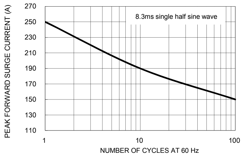
FIG. 7 MAXIMUM NON-REPETITIVE PEAK FORWARD SURGE CURRENT
