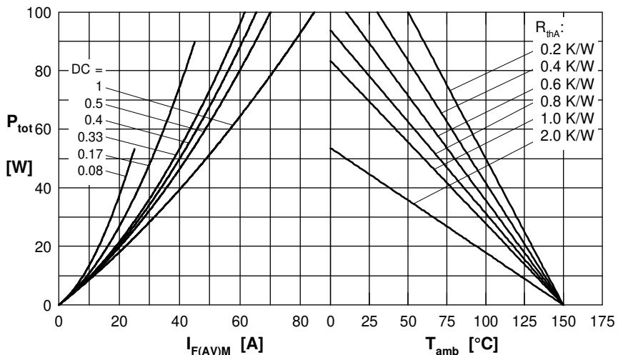
Fig. 4 Power dissipation vs. forward current
