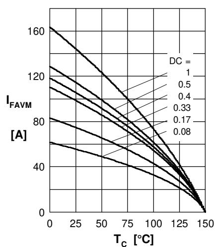
Fig. 5 Max. forward current vs.
