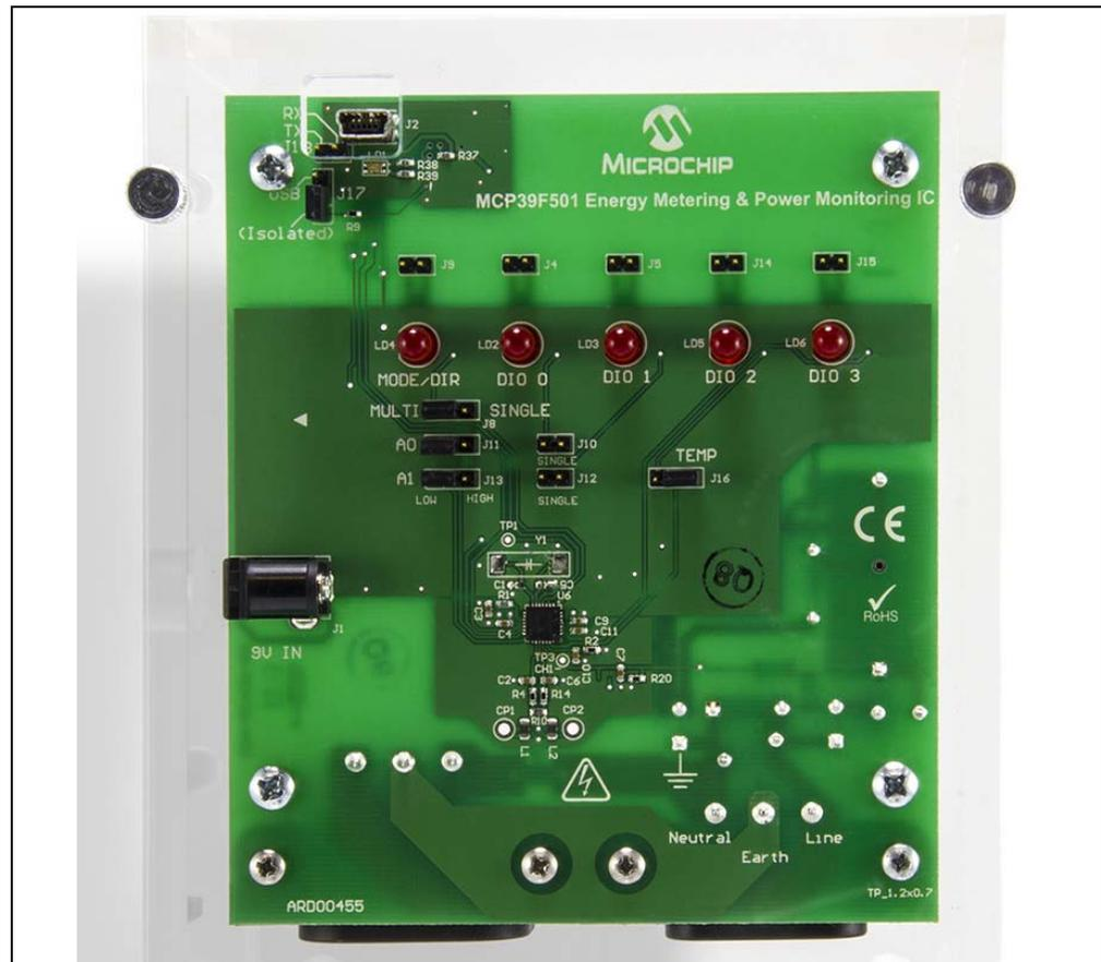
**FIGURE 1-1:** MCP39F501 Power Monitor Demonstration Board.
