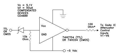
Simple driver using inexpensive standard logic ICs provides fast switching using minimum DC current. \* Recommended value to suppress unwanted RF signals at V1 -V6 control lines.
