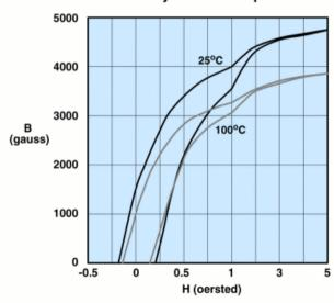
Measured on an 18/10/6mm toroid at 10kHz.
