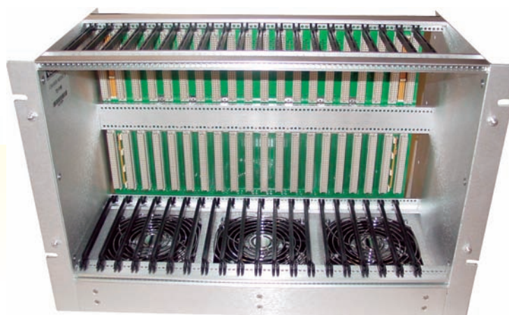
VectorPak™ powered subrack with VME J1/J2 backplane and integrated fans
