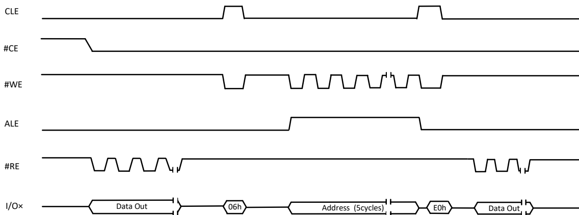
Figure 9-4 Two Plane Random Data Read (06h-E0h) Operation
