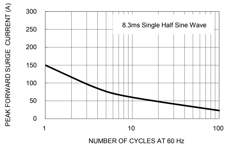
FIG. 2 MAXIMUM NON-REPETITIVE FORWARD SURGE CURRENT PER LEG
