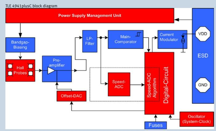
The TLE4941 plus C signal path includes a pair of hall probes (2 mm spacing), a differential amplifier and a comparator feeding a switched current output stage. Additionally, the circuit has a feedback loop for offset compensation which consists of a signal-Speed ADC, a digital signal processor (DSP) and an offset D/A converter.
