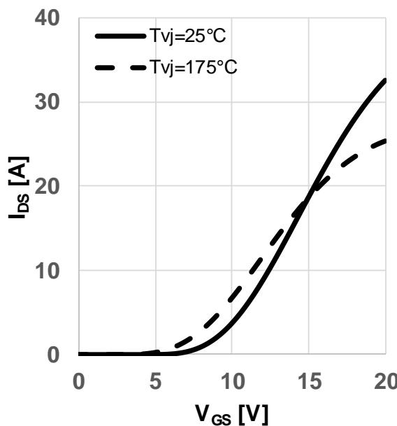
**Figure 5** Typical transfer characteristic
