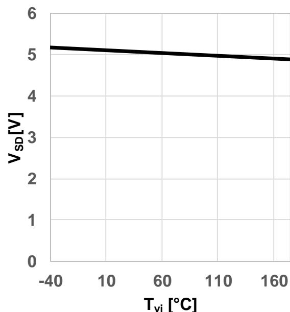
**Figure 12** Typical body diode forward voltage as function of junction temperature
