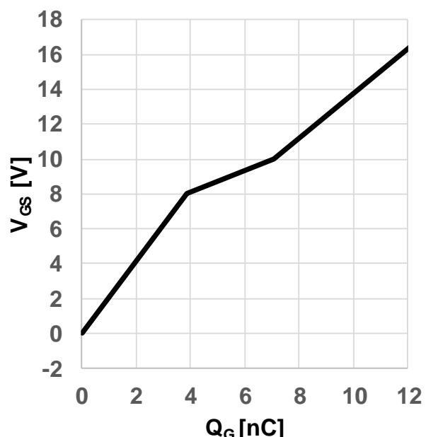
**Figure 10** Typical gate charge
