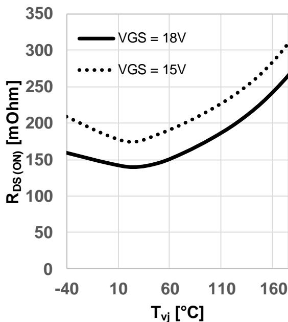
**Figure 9** Typical on-resistance as a function of junction temperature
