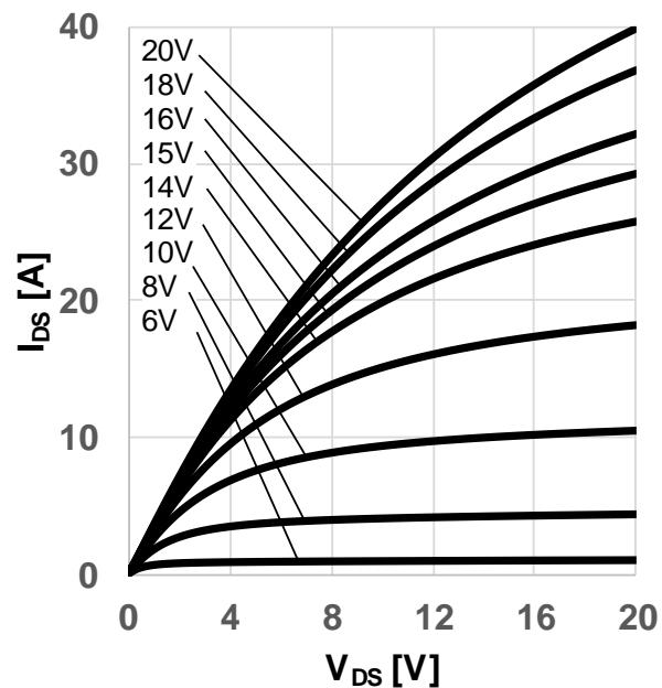
**Figure 8** Typical output characteristic,  $V_{GS}$  as parameter
