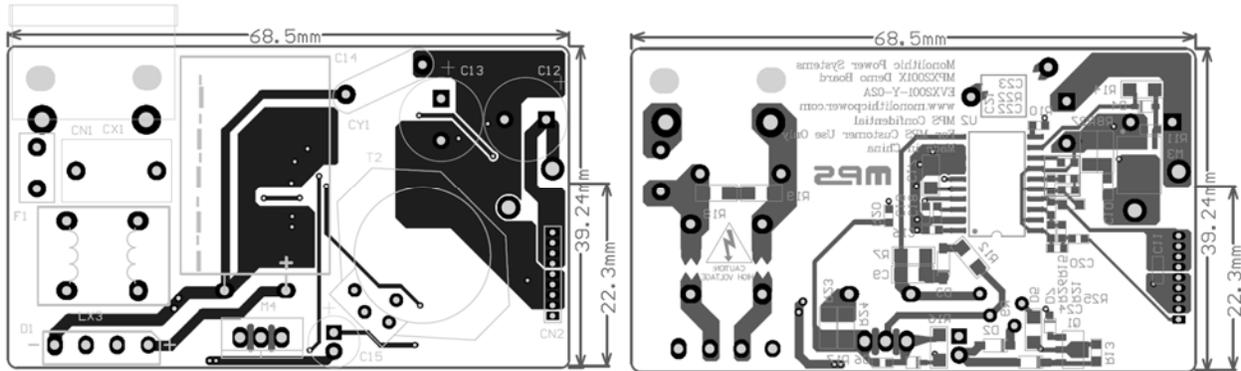
Figure 14: Top and Bottom Layer of Main Board
