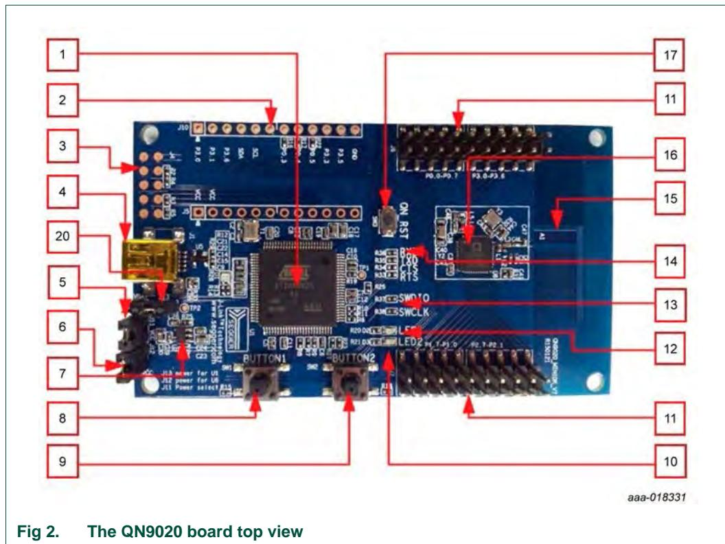
**Fig 2.** The QN9020 board top view
