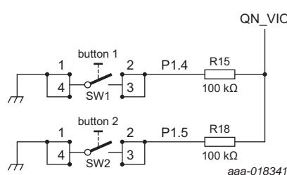
Fig 13. Button circuit
