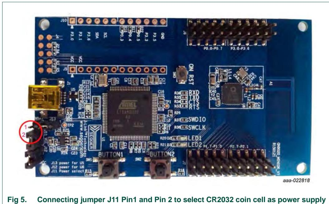
Fig 5. Connecting jumper J11 Pin1 and Pin 2 to select CR2032 coin cell as power supply
