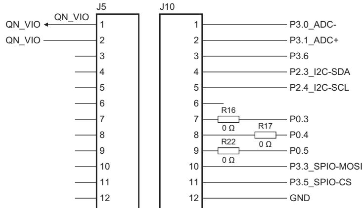
**Fig 15. Connecting the sensor board**
