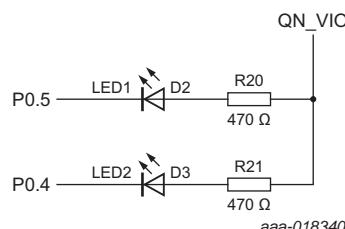
Fig 12. LED circuit
