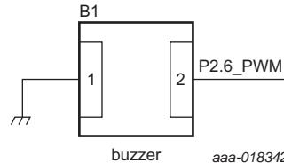
**Fig 14. Piezo buzzer circuit**
