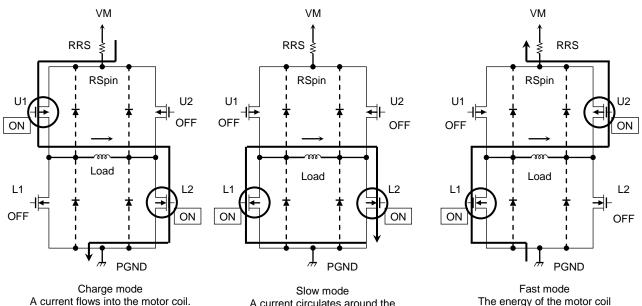
A current circulates around the motor coil and this device.
