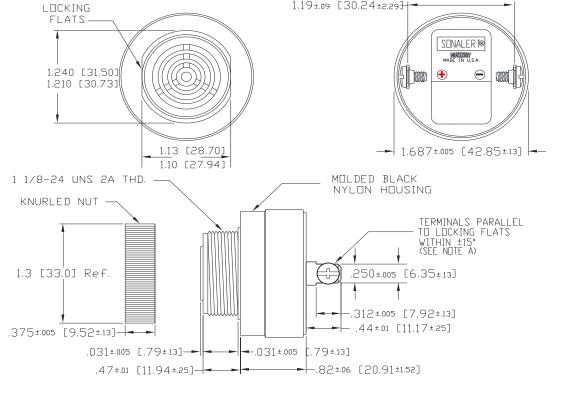
NOTE A: TERMINALS-.032 BRASS TIN PLATED, TAPPED FOR #6-32 SCREW. TWO #6-32 NICKEL PLATED BRASS SCREWS INCLUDED. WILL ACCEPT 1/4" QUICK CONNECT. NOTE B: MOUNTING- REMOVE BLACK PLASTIC NUT AND INSERT THREADED FRONT THROUGH 1.25" HOLE PUNCHED IN PANEL, IF DRIENTATION IS NEEDED, NOTE LOCKING FLATS ON DRAWING. SCREW NUT BACK ON. DO NOT OVERTIGHTEN.
