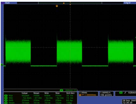
FIGURE 11. I L AT 50% PWM DIMMING
