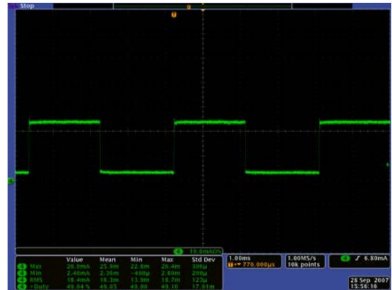
FIGURE 16. I LED AT 50% PWM DIMMING
