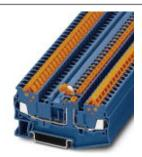
Feed-through terminal block, Connection type: Quick connection, Cross section: 0.25 mm² - 1.5 mm², AWG: 24 - 16, Nominal current: 17.5 A, Nominal voltage: 400 V, Length: 76.4 mm, Width: 5.2 mm, Color: blue, Assembly: NS 35/7,5, NS 35/15
