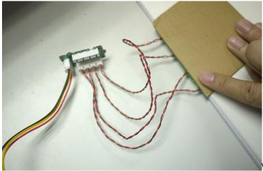
With a paperboard about 3 mm thick, the feeler can feel the touch of fingers, makes it a good solution for many applications.
