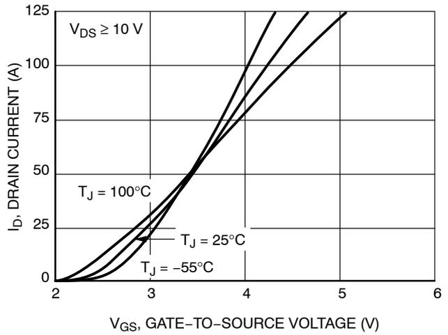
Figure 2. Transfer Characteristics
