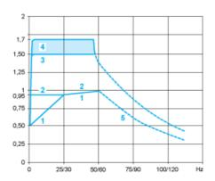
1: Self-cooled motor: continuous useful torque (1)
