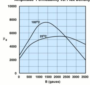
Measured on an 18/10/6mm toroid at 10kHz.
