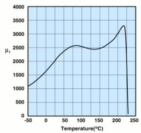
Measured on an 18/10/6mm toroid at 100kHz.
