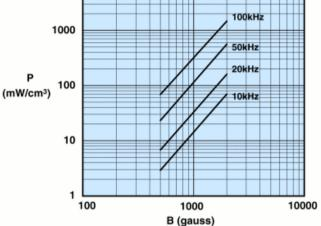
Measured on an 18/10/6mm toroid using the Clarke Hess 258 VAW at 100°C
