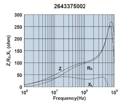
Impedance, reactance, and resistance vs. frequency.
