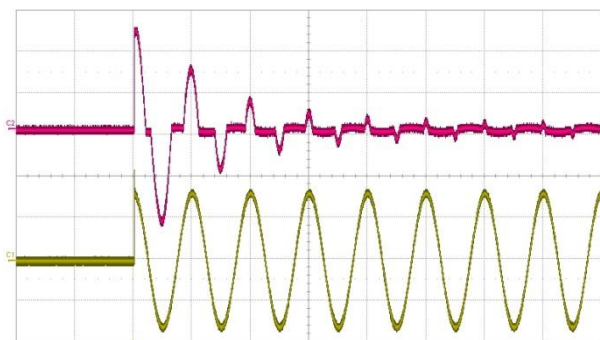
Figure 4: Inrush current, V_{in} = 230\ V_{ac}, 90^\circ CH1: V_{in} (200 V/div), CH2: I_{in} (5 A/div)
