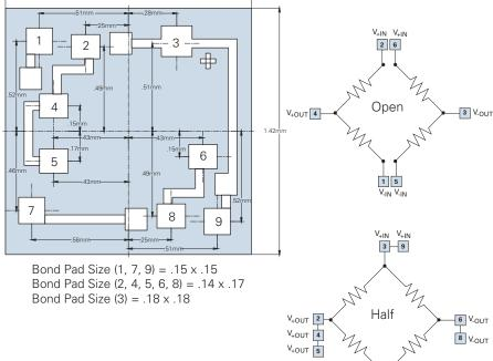
Note: Bridge output bond pads ( $V_{\text{-out}}$  and  $V_{\text{+out}}$ )correspond to top side pressure. For back side pressure, the bridge outputs are reversed.
