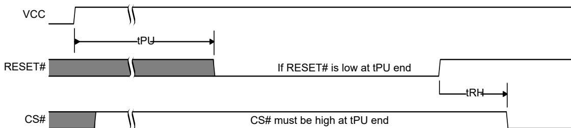
Figure 136. Reset low at the end of POR
